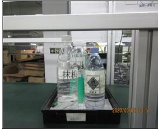
Photo of non-conformity Chemical containers used at workshop were not posted suitable chemical labels.JPG
