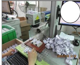
Photo of the inside of the main production hall LEV for laser carving.JPG
